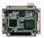
Portwell PEM-P393 is a PC/104-PLUS single board computer which uses Intel® Pineview N455 single core 1.66 GHz processor paired with the ICH8M I/O controller hub. It includes one SODIMM socket for DDR3 system memory and one Compact Flash socket.
