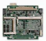
The PC/104-PLUS module is a full-featured unit with on-board I/O that supports CRT/LVDS simultaneously, Gigabit Ethernet port, eight USB 2.0 ports, four RS232 (two 422 /485 selectable COM channels), 24 digital I/O lines with event sense, HD audio and a watchdog timer. Additionally, it has a PC/104-Plus connectors for I/O expansion. The low power, high performance and fan-less requirement, it is suitable for Automation, Medical, Transportation, Security, Military and HMI applications.
