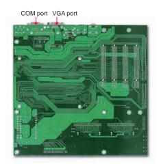
Portwell PEM-C200 is designed with ETX connector type released by ETX industrial group, suitable for initial evaluation testing in PCI, ISA, VGA/LVDS, IDE, LAN, USB, Serial, Parallel, AUDIO, etc. interfaces before developing your own application focused customized carrier board.
