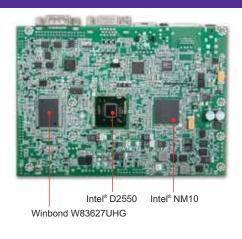
PEB-2772 takes advantage of the processor's performance and furthermore Portwell design the CPU/chipset on the backside of the board which is good for system thermal design. Customer could take this advantage to have an easy and perfect thermal solution which could solve the thermal of CPU.
