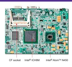
The PEB-2770/2780 takes advange of the latest Intel® Atom™ technologies. It supports DDR2 SDRAM, dual gigabit ethernet and one expansion PCI Express x1 female header. Based on Intel® Atom™ solutions, the fanless PEB-2770/2780 executes high performance with low power dissipation. Therefore, it's applied to Panel PC, Kiosk, DS, Medical, Military and industrial automation.
