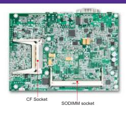
The PEB-2739I takes advange of the latest Intel® Atom™ technologies. It supports DDR2 SDRAM, one gigabit ethernet and one expansion Multi function connector. Based on Intel® Atom™ solutions, the fanless PEB-2739I executes high performance with low power dissipation. Therefore, it's applied to Panel PC, Kiosk, Medical, and industrial automation.
