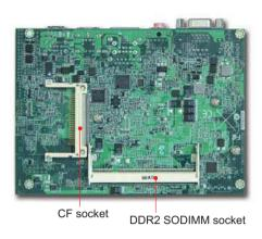
PEB-2737VLA takes advange of the latest Intel® Atom™ technologies. It supports DDR2 SDRAM, and one gigabit ethernet. Based on Intel® Atom™ solutions, the fanless PEB-2737VLA executes high performance with low power dissipation. Therefore, making it the ideal solution for Panel PCs, Kiosks, and Industrial Automation.
