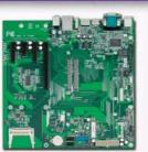
Micro-ATX Form Factor Evaluation Carrier Board For COM-Express Revision 2.0 Type VI Module.
