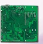
Portwell PCOM-C600 is designed with Micro-ATX form factor with COM Express Type VI row connectors, suitable for evaluation testing of Portwell's Type 6 & 10 COM Express modules on USB3.0.PCI-E (x16, x4, x1, ADD2) Mini-PCI-E, mSATA, PEG/SDVO, HDMI, DVI, LVDS, DP, SATA, LAN, AUDIO etc. We also provide carrier board design guides for your own carrier board development reference.
