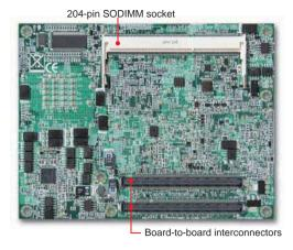
Portwell PCOM-B213VG is designed with GM45 and ICH9M chipset, with improved Intel® Gen 5 graphic engine that included advance HDMI, display port interfaces suitable for medical, media, gaming and infotainment applications, and featuring with DDR3, iAMT 4.0, and TPM for effective security for remote application like network, communication and industrial control.
