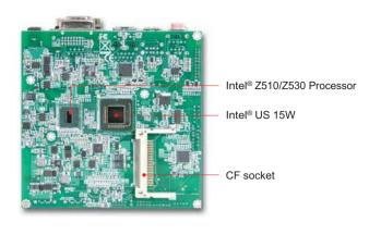
NANO-8045 takes advantage of the latest Intel® Atom $^{\text{TM}}$  technologies. It supports DDR2 SDRAM, dual displays and one Gigabit Ethernet. Based on leading edge Intel® Atom™ solution, NANO-8045 is compact with a low power dissipation board ready for Medical, Mobile, Gaming, and DS applications.
