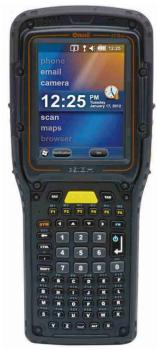
The Omnii XT15ni is a modular industrial handheld computer, that is UL-certified to be non-incendive, which ensures safe operation in hazardous areas found in pharmaceutical, oil & gas, utilities, chemical, and various manufacturing applications. The XT15ni features a variety of options including imagers, RFID, Push-to-Talk speaker, camera, WAN radio and keyboards.
