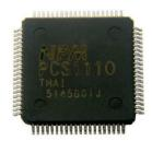
Also possible is the utilization of more than one PCS1110 chip which allows for multiple independent electronic 'slave' cam control off of one 'master' motion profile, an impossibility with a mechanical cam.
