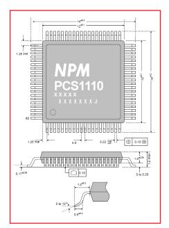
The PCS1110 is a programmable pulse generator designed to replace a mechanical cam. The first of its kind, the PCS1110 chip controls a secondary axis, moving to the target position in direct relation with the main axis, just as a mechanical cam would perform.
