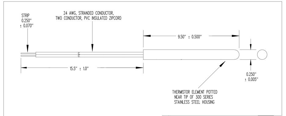
RESISTANCE  $\[Omega]$  +25°C = 100,000  $\[Omega]$  NOMINAL ACCURACY (0 TO +105°C) =  $\pm$  0.01°C OF R-T CHART SUPPLIED WITH PROBE RESISTANCE/TEMPERATURE CURVE = "J" BETA " $\[Omega]$ " (0 TO +50°C) = 3,892°K NOMINAL TEMPERATURE COEFFICIENT  $\[Omega]$  +25°C = -4.4%/°C NOMINAL TYPICAL DRIFT: <0.01°C/YEAR MAXIMUM TEMPERATURE RATING = +105°C
