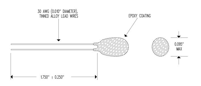
RESISTANCE @  $+25^{\circ}C = 50,000 \Omega$  NOMINAL ACCURACY (0 TO  $+50^{\circ}$ C) =  $\pm 0.05^{\circ}$ C RESISTANCE/TEMPERATURE CURVE = "J" TEMPERATURE COEFFICIENT @  $+25^{\circ}C = -4.4\%$ /C NOMINAL
