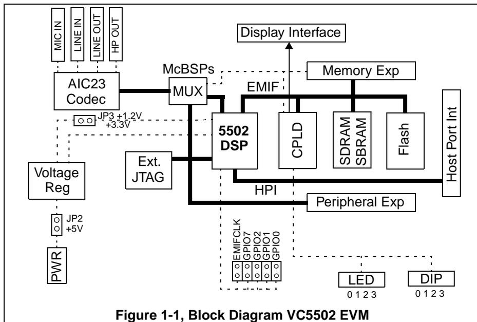
Figure 1-1, Block Diagram VC5502 EVM
