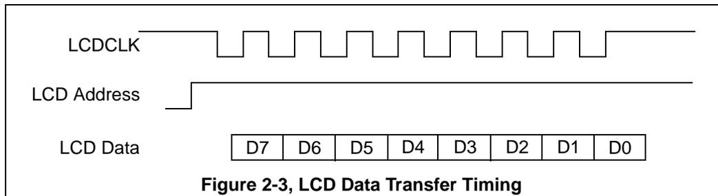
After any write operations the CPLD sets the LCD BUSY bit in the VC5502 EVM interface Register as the output is being serialized. The user should check this bit prior to starting another write operation. When LCD BUSY is high, the LCD shift register is busy, when is low the shift register is ready.
