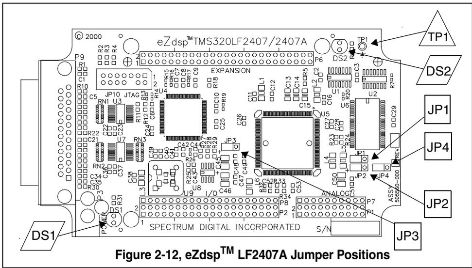
**Figure 2-12, eZdsp™ LF2407A Jumper Positions**
