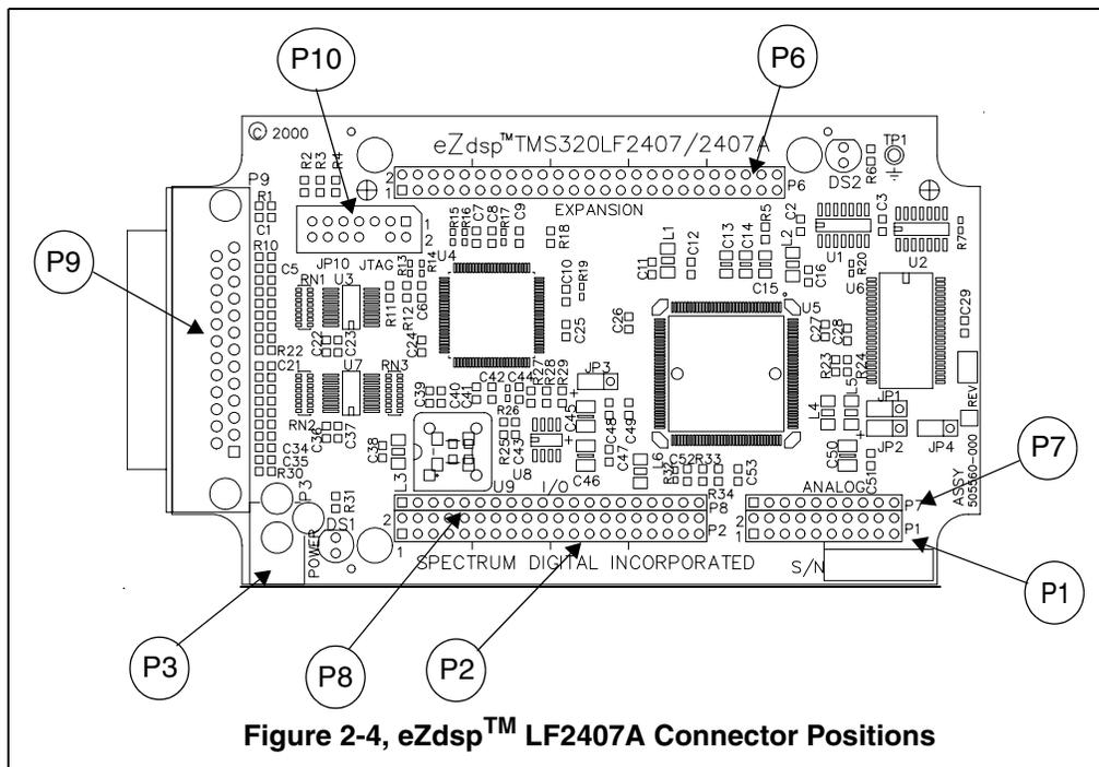
**Figure 2-4, eZdsp™ LF2407A Connector Positions**
