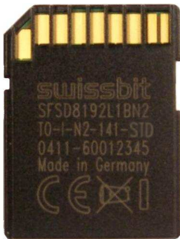
Example of the back side laser marking
