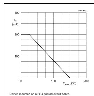
Fig.2 Maximum permissible continuous forward current as a function of ambient
