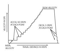
The separate decelerate parameter is a valuable time saver when compared to systems with fixe d acceleration and deceleration times.
