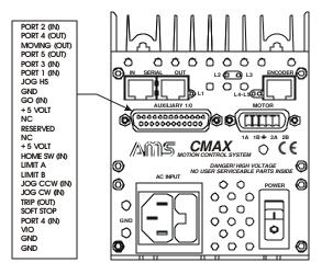
All inputs have RC noise filters, followed by voltage comparators with hysteresis, for high noise immunity. The input threshold voltage is set to 50% of VIO, the input circuit supply voltage. VIO is supplied from the 6 volt bias supply via an isolation diode. An external supply may be used if a higher input voltage
