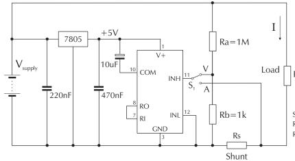
$S_1$  selects between voltage and current display. Ra and Rb shown scaled for  $200V_{FSR}$ .
