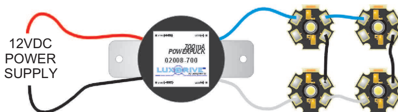
PowerPuck 2008-700 driving (4) Luxeon I LEDs from 12VDC.
