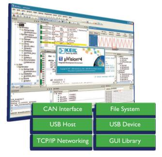
Keil<sup>™</sup> MDK-ARM<sup>™</sup> (Microcontroller Development Kit) the complete software development environment for ARM processor-based microcontrollers.
