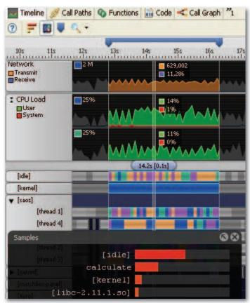
**Timeline view** shows process and thread information over time, matched to SoC performance counters. This enables visibility of spot thread deadlocks and inefficiencies, as well as hot spots in time.
