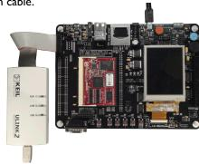
ULINK2 supports the Keil Real-Time Agent for "on-the-fly" debug of running applications via the JTAG port.
