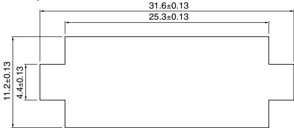
Note: 1. Punch holes in the panel according to the sketch and table shown above. Burrs must be removed.
