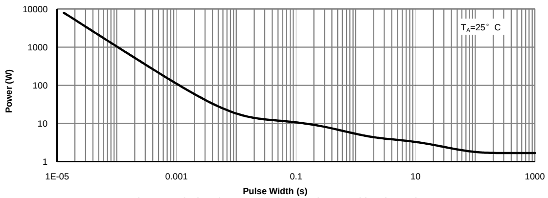
Figure 14: Single Pulse Power Rating Junction-to-Ambient (Note H)
