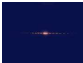
Figure 5. Diffraction pattern created by two razor blades.
