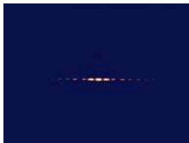
Figure 6. Laser diffraction pattern from dual slit.
