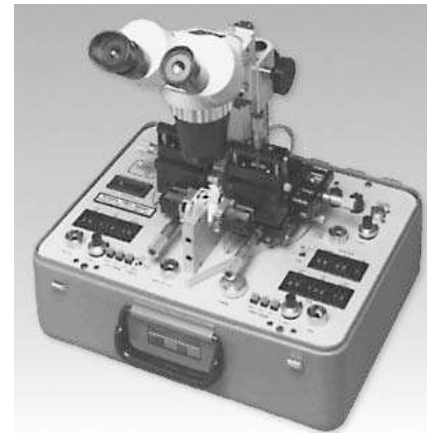
Photo 20. Fusion splice for glass optical fiber.
