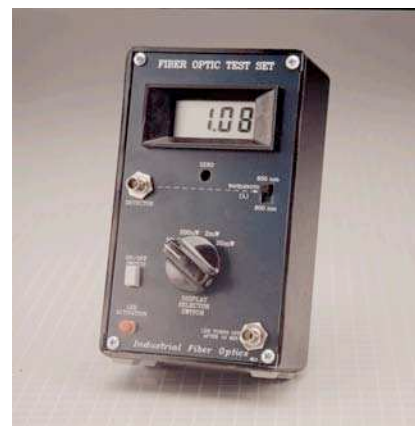
Photo 21. Optical power meter with a built-in light source.
