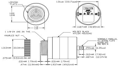
NOTE A TERMINALS-.032 BRASS TIN PLATED, TAPPED FOR #6-32 SCREW. TWO #6-32 NICKEL PLATED BRASS SCREWS INCLUBED. WILL ACCEPT 1/4' QUICK CONNECT.
