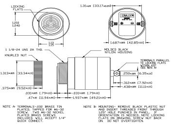
NDTE BI MUUNTING- REMOVE BLACK PLASTIC NUT AND INSERT THREADED FRONT THROUGH 1.25' HOLE PUNCHED IN PANEL, IF DRIENTATION IS NEEDED, NOTE LOCKING FLATS ON DRAWING, SCREW NUT BACK ON. DO NOT OVERTIGHTEN.
