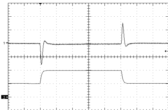
Figure 13. Load Transient Response (100mV/div), di/dt=0.1A/uS, 50% - 25% - 50% of full load, time scale: 200uS/div.
