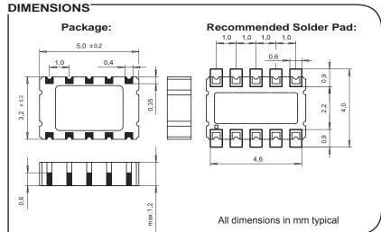
Extremely Accurate RTC Module with embedded Xtal. I<sup>2</sup>C Interface Temperature Compensation Automotive qualified, according to AEC-Q200 Rev. C
