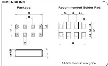
Ultra small SMT ceramic package with integrated 32.768kHz Crystal Automotive qualified, according to AEC-Q200 Rev. C I<sup>2</sup>C Interface Address: D0h Frequency-Offset Trimming Register Programmable Alarm and Interrupt Oscillator Fail Detection Watchdog Timer Programmable Clock-Output Time keeping mode down to 1.0 V
