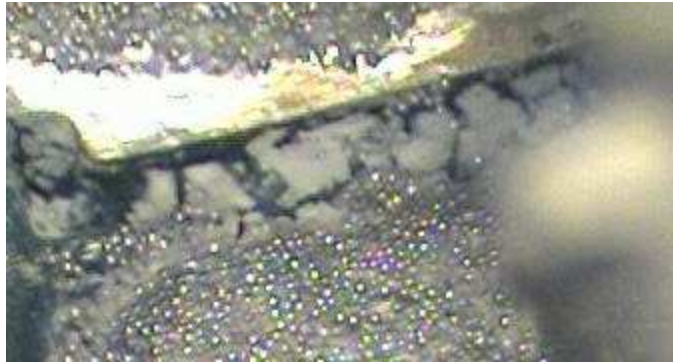
Figure 4: Unacceptable - White residue between the leads
