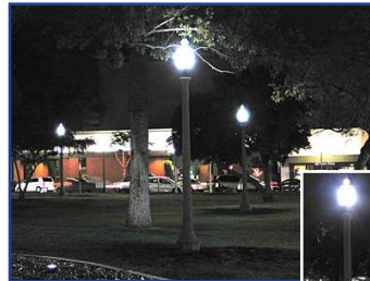
Above and at right, LED30MH-600 bulbs replace 150W globe bulbs in Library Park in Monrovia, California.
