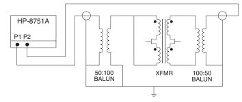
5. Crosstalk Attentuation - In the packages which contain transmit and receive transformers side by side, sufficient crosstalk attentuation is achieved by the inherent characteristics of the toroid cores as well as by their proper positioning. The crosstalk attentuation is typically 65 dB or better. This result was established with the test circuit shown below.
