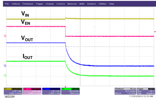
Enable OFF Sequence ( R_L=8\Omega ) VEN=2V to 0V
