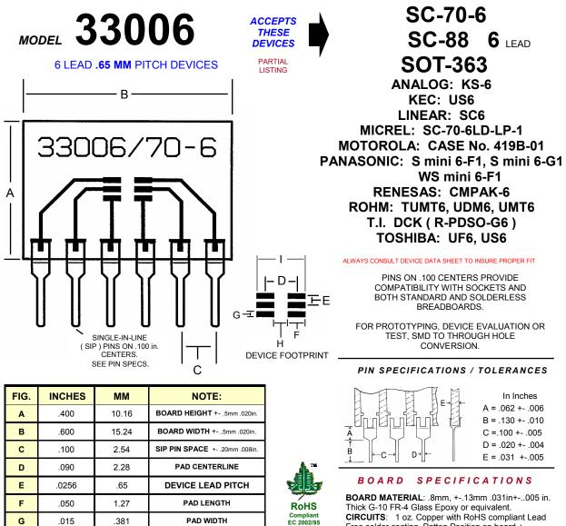
CIRCUITS: 1 oz. Copper with RoHS compliant Lead Free solder coating. Patten Position on board +-.5mm .020in.
