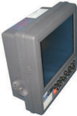
In compliance with the latest IMO regulations the AE-2000 features two independently operating receivers. These receivers allow for the simultaneous reception of the standard 518 KHz NAVTEX signal, and either the 490 KHz or 4,209.5 KHz that is broadcast in some
