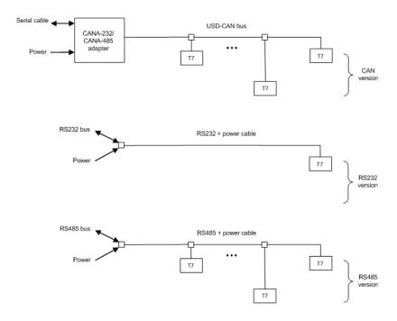
US Digital sells all the cables and connectors needed to wire a T7 network. The T7 uses the same connector for all interface versions.
