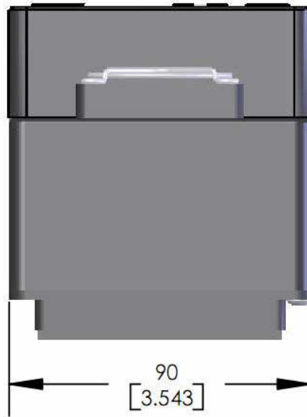
Figure 11: Standard Body (Type A) with Rectangular Flange (Type A) - Top View
