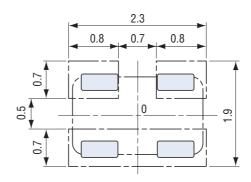
Note) The zero point is center of mounting
