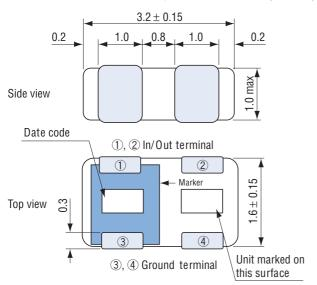
**E-TA2012** Unless otherwise specified, tolerance : ± 0.2 (Unit : mm)
