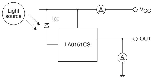
\*4. Measuring method of rise time ( $T_r$ ) and fall time ( $T_f$ )
