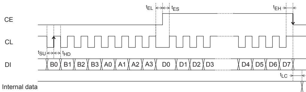
**Serial data output (OUT)** tSU, tHD, tEL, tES, tEH $\geq$ 0.75μs tDC, tDH<0.35μs
