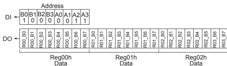
"C1" is input from LSB to the start as an address when the serial data is output from LV23401V, the controlled device is specified, and the mode as the data output is fixed. The subsequent data is output from DO pin synchronizing with lock (CL) after the address is input LSB from one with small register number. The output of data is ended by setting CE pin to Low.
