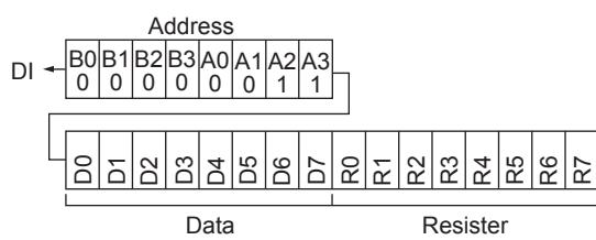
LV23401V is controlled by the bus format composed of the sub-address (register) that stores the data of the device address of 8bit (address) and each 8bit. "C0" is input from LSB to the start as an address when the serial data is input to LV23401V, the device that controls is specified, and the mode as the data input is fixed. It inputs from LSB in order of data (bit setting) → register synchronizing with data clock (CL) after the address is input and the data input can be concluded.
