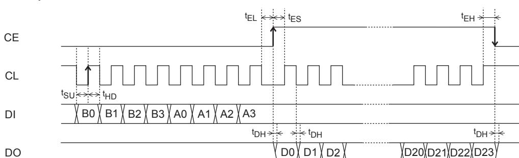
(Note) DO pin is an Nch open drain pin, so that the data varying time (tDC and tDH) differs depending on the pull-up resistance and substrate capacity.
