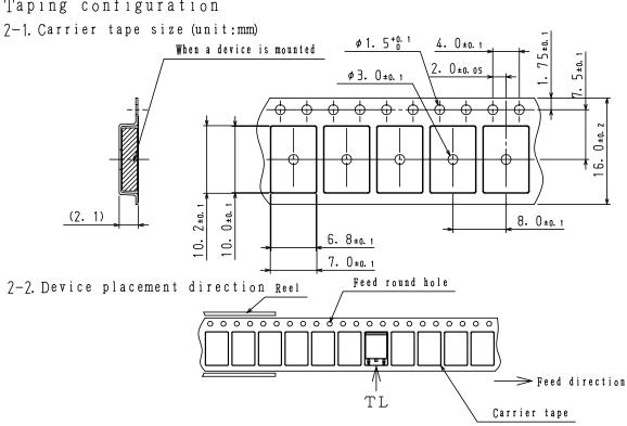
The one erectrode terminals on feed hole side····TL
