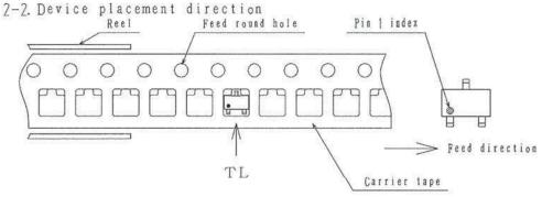
Those with one electrode terminal on the feed hole side.....TL
