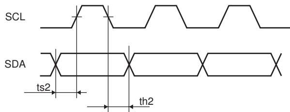
When data is not being transferred, both SCL and SDA are in the high state. The start condition is generated and access is started when SDA is changed from high to low while SCL and SDA are high.
