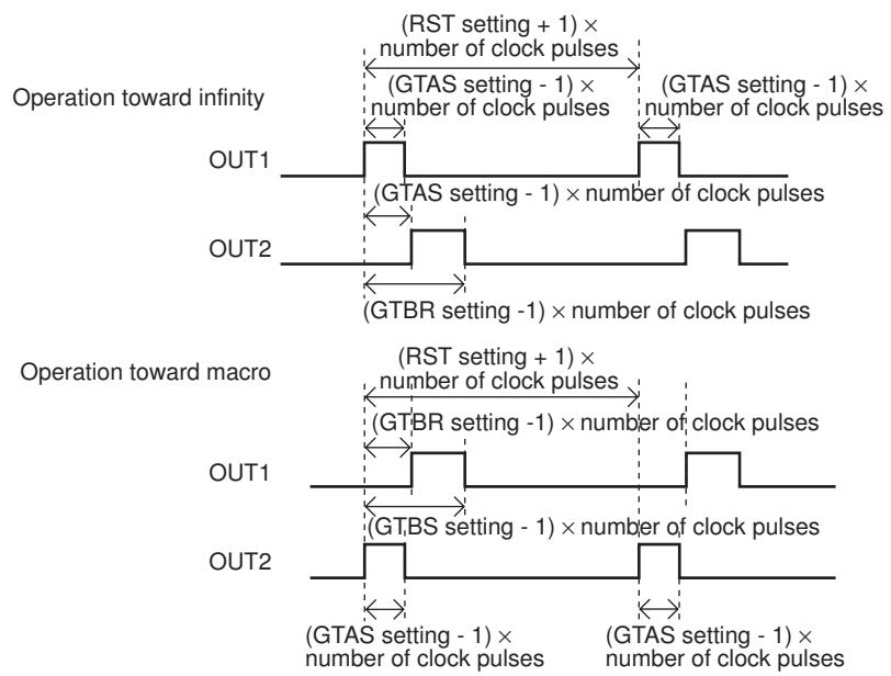
Sequence of initial setting operation (“on” or “off” can be set by the I<sup>2</sup>C settings.)
