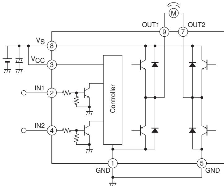
Note: When using the same power supply for V<sub>S</sub> and V<sub>CC</sub>, short the V<sub>CC</sub> and V<sub>S</sub> pins to each other or insert a capacitor in the V<sub>CC</sub> line.
