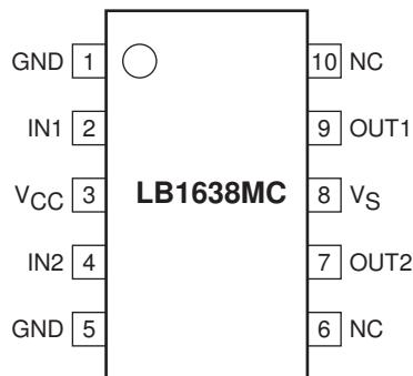
Note: both ground pins must be grounded.
