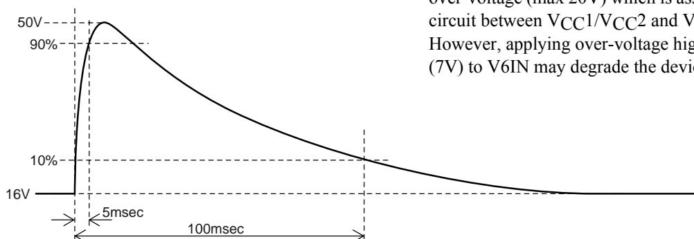
\*V6IN is designed to tolerant toward short period of over-voltage (max 20V) which is assumed in condition of short circuit between  $V_{CC1}/V_{CC2}$  and V6IN. However, applying over-voltage higher than maximum rating (7V) to V6IN may degrade the device reliability
