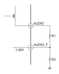
The AUDIO\_F voltage is determined by the internal band gap voltage of the IC (typ = 1.26V).
