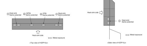
• Frame diagram (LV5680NPVC) \*In the system power supply other than LV5680NPVC, pin assignment may differ.
