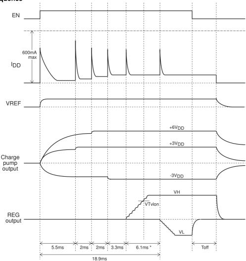
\*The VL startup time at VH ≥ 10V and after elapse of 6.1ms is the reference time for CLK = 2MHz.
